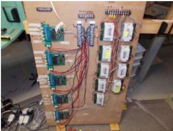
The switches are finished to the extent of the electronic switches we have. Of course there are still kinks and headaches of a 20 year old layout with the turnouts and track. To date, six turnouts that aren't throwing reliably as we would like, however we have 35 turnouts operating as they should. Overall this is minor stuff that we can work around until time and manpower is available for repairs. There are also few places, on and off mainlines, of track that should be repaired.
